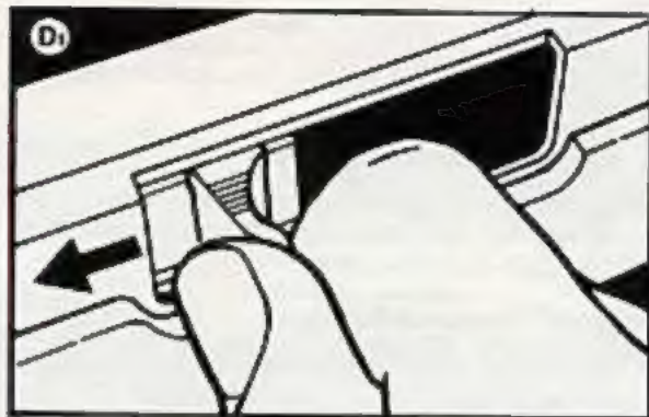
Pull charging handle all the way back.
